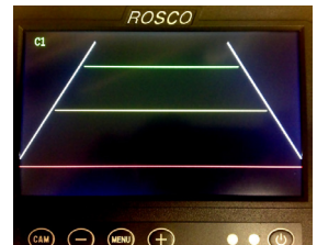
Appearance of the Backup Grid
