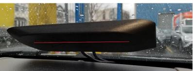
Fig 3. Bottom Side Windshield Mount Antenna (Interior View)
