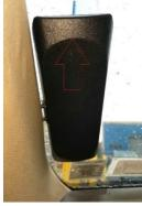
Fig 1. Left Side Windshield Mount Antenna (Interior View)
