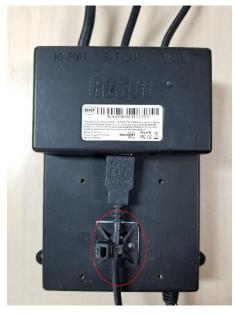
Fig 6. Use a zip tie (TIE1001) and secure the USB cable on PDC
