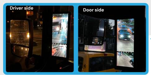
The images on the left show a comparison of standard rearview mirrors to the D•CAMS monitors in low light conditions on both the driver's side and door side of the vehicle.
