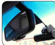
Adjust Camera Lens for Best Viewing Angle
