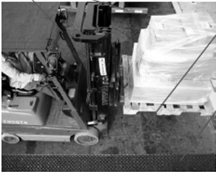
Typical monitor image of view from properly installed camera
